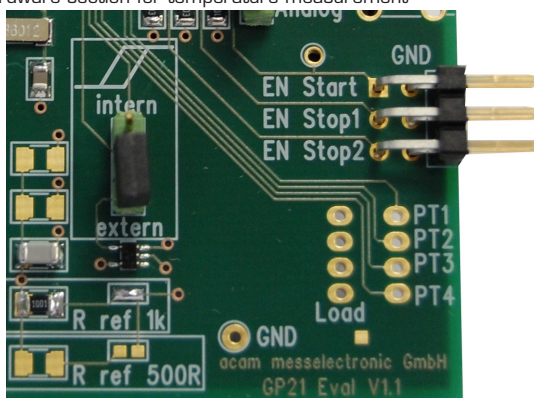
Figure 2.14: Hardware section for temperature measurement
