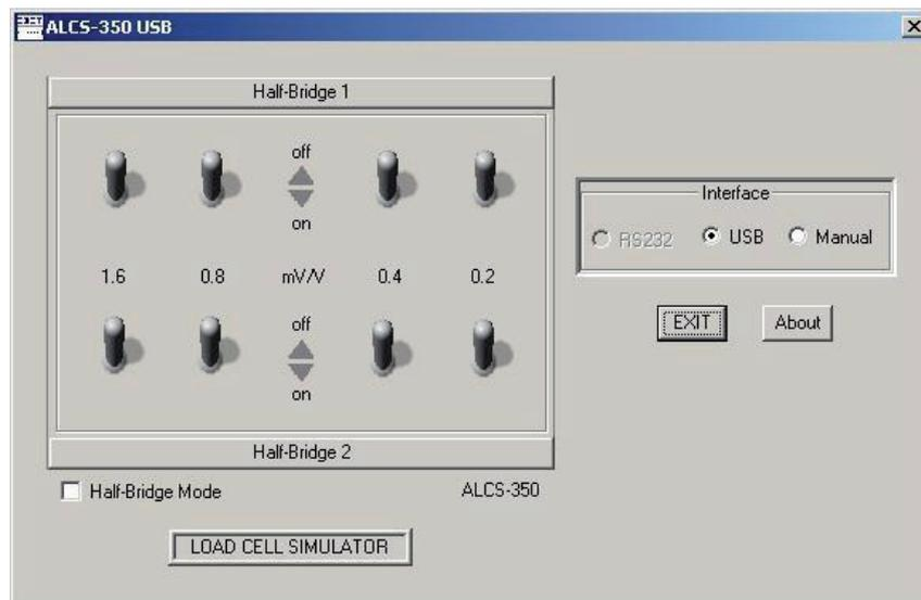
By default the user software runs in Wheatstone or full bridge mode. The corresponding switches on rows half bridge 1 and 2 are tied together and change simultaneously. So the same strain is simulated on both bridges arms.
