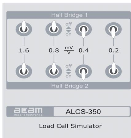
The simulated strain is set separately and in the opposite direction for the two bridge arms. This way the simulated strain can be set from 0 to 3 mV/V in steps of 0.1 mV/V in full bridge mode or 0.2 mV/V in half bridge mode.
