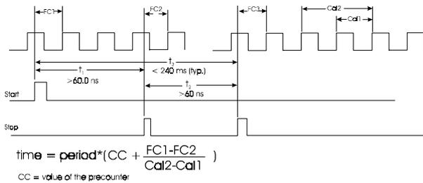
The minimum measurement time is given as two cycles of the reference clock. The maximum measurement time is given as 2<sup>16</sup> times the cycle of the reference clock and can reach 200ms.
